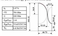
Figure 5: Parameters and dimensions (in mm) of the optimized regular cell. Lorentz factor  $K_L$  is given for optimal stiffening ring.
