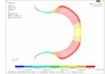
b) With the ring,  $K_L=0.43 \text{ Hz/(MeV/m}^{)2}$
