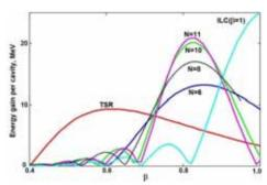
Figure 7: The energy gain per cavity versus  $\beta$  for the  $\beta$ =0.81 cavities with different number of cells. The surface peak electric field is 50 MV/m.
