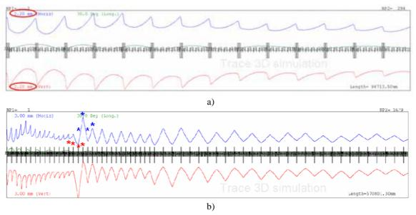
Figure 3: The beam envelope in S-ILC section (a) and S-ILC matching to the ILC1 (b). Blue – horizontal, red – vertical, green – longitudinal r.m.s. size in deg. Stars show the elements used for matching.
