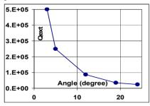
Figure 9: Loaded Q – factor for the operating mode versus the couler orientation angle.
