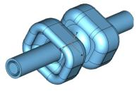
Figure 3: Initial version of the mushroom crab cavity with the coaxial couplers. Horizontal size is 350 mm. For the kick of 2.5 MV  $E_{peak}$ =36.6 MV/m and  $H_{peak}$ =135 mT.
