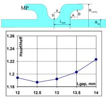
Figure 5: The cavity optimization in 2D approximation. The cavity cross section (top) and maximal surface magnetic field vs. gap length (bottom).
