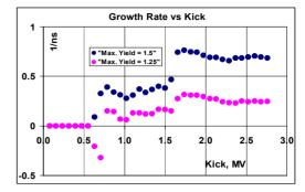
Figure 10: Growth rate of MP vs. kick for different secondary emission yield functions (Maximum 1.5 and 1.25 respectively.
