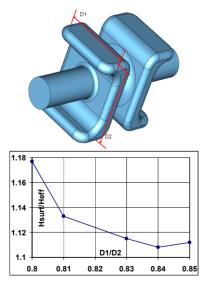
Figure 6: 3D cavity shape optimization.
