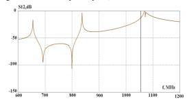
Figure 8: The SOM coupler: S<sub>12</sub> versus frequency
