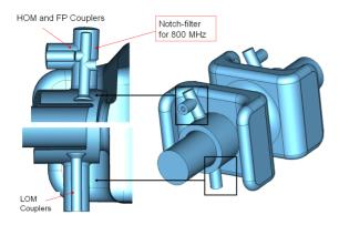
Figure 4: 2-cell mushroom crab cavity design with the coaxial coupler units at the cavity ends.
