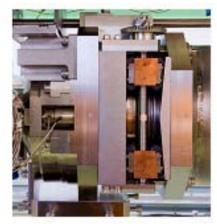
Figure 7: Slide jack tuner.
