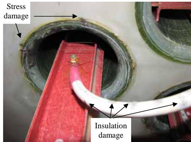
Figure 5: Electrical damage on silicone-insulated lead and stress damage at dielectric-to-dielectric interface.
