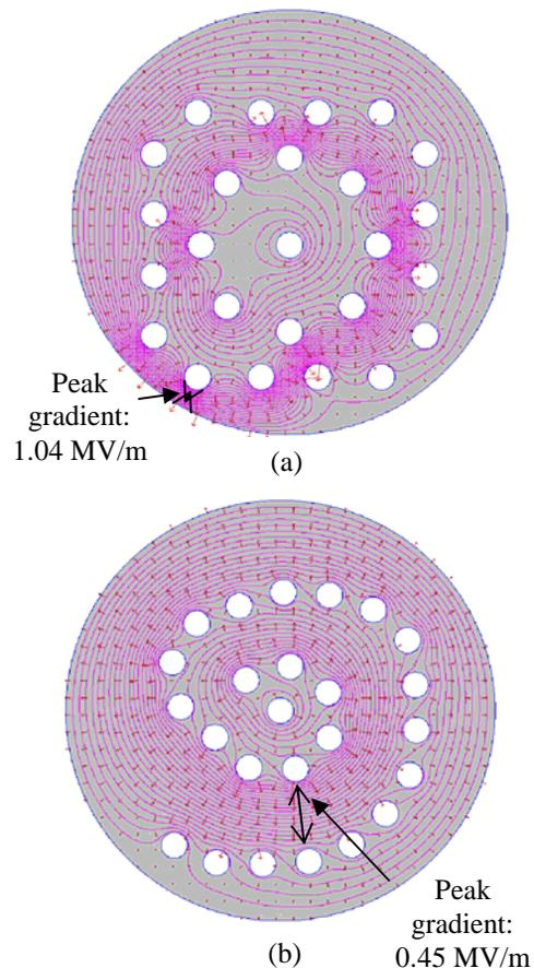
Figure 1: Electrical field contours of the (a) original and (b) redesigned load geometries using Poisson solver. The peak voltage level is 100 kV and is located in the center of each of the designs. A 4-kV voltage drop exists across each resistor, and the outer radius of the containment vessel is assumed to be grounded. A path along which the peak gradient exists is shown for each of the load designs.
