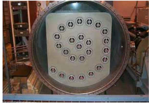
Figure 3: Internal view of the redesigned load with the resistor network and dielectric structures.
