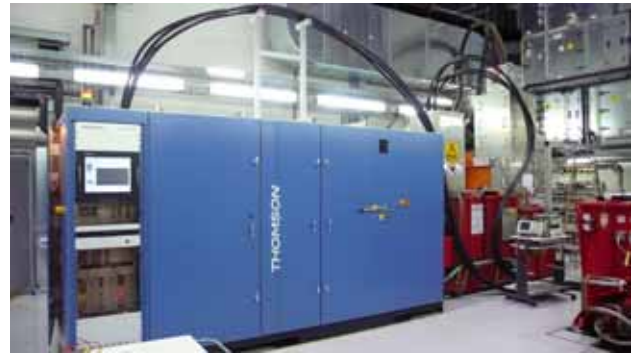
Figure 3: The Thomson modulator in the MTF hall.
