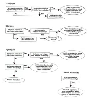
Figure 1: Flow Chart for the Key Gas Analysis [2].
