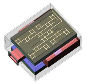
Figure 2: Strip line RF power adder.
