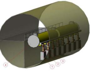
Figure 5: Accelerator module with Solid State High Power RF System in XFEL tunnel.
