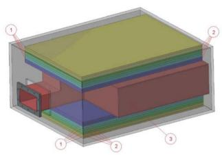
Figure 4: General view of Solid State Generator. 1 is amplifier unit, 2 is strip line RF power adder, 3 is waveguide RF power adder.
