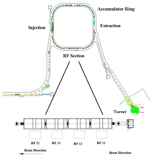
Figure 2: Layout of ring RF components.
