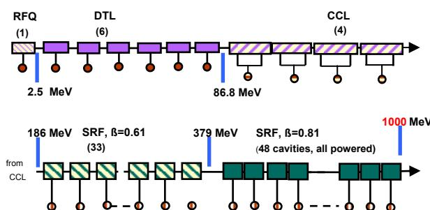
Figure 1: Layout of LINAC RF modules.
