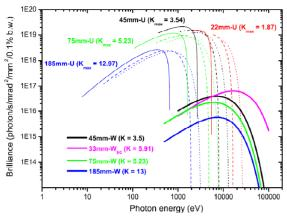
Figure 5. Brilliance of synchrotron radiation emitted from the undulators and wigglers at the TAC positron ring.
