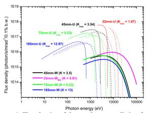
Figure 4. Flux density of the synchrotron radiation from IDs
