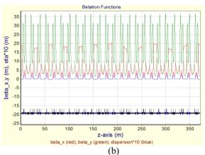
Figure 3. Optics at the storage ring: (a) without IDs, (b) with five IDs.
