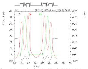
Figure 1. Lattice functions for 12 period DDBA lattice
