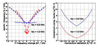
Figure 3: Left: Synchrotron frequency  $f_s$  as a function of the rf-frequency change  $\Delta f_{rf}$  for two different sets of  $\alpha$ ,  $\alpha_0 = 8.25E - 5$  and  $\alpha_0 = 4.6E - 4$ . The circles show measurements with octupole 'off', the square data with octupole 'on'. Right: Nonlinear  $\alpha$  as a function of momentum deviation  $\delta$ . Both Figures apply the data with octupoles 'on'.
