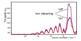
Figure 4: Detected Fourier-Transform THz spectrum with and without applied ion clearing voltage. The low frequency part of the spectrum doubles intensiy if the clearing voltage is switched off.
