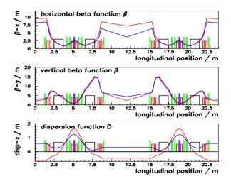
Figure 1: Optical functions of the user optics (blue line) and the  $\alpha = 0$  optics (red line). Half of the ring is displayed. Magnetic multipoles are indicated by coloured boxes, dipoles (black), quadrupoles (red), sextupoles (green), octupoles (blue).
