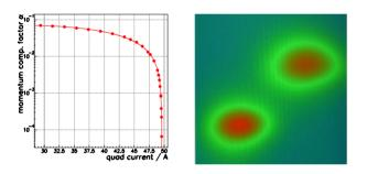
Figure 2: Left: The low- $\alpha$  tuning range ( $\alpha_0 > 0$ ) of the MLS at 630 MeV as a function of the quadrupole 'q1' current (dots). The trend line is a parabolic fit to the data. Right: If  $\alpha_0$  becomes < 0 the beam splits into a stable pair of  $\alpha$ -buckets, visible on a synchrotron radiation monitor.
