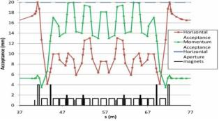
Figure 5: Horizontal and momentum acceptance for one quarter of the booster. Limiting apertures are in the second quadrupole and the second focusing dipole.
