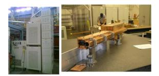
Figure 1: Example of newly installed or upgraded hardware: New booster bend magnet power supply; upgraded septum magnet.
