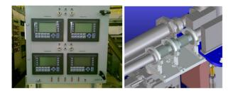
Figure 2: Left: Example of newly installed interlock system - PLC chassis, which are part of the beam current, lattice, and energy match interlocks. Right: Example of newly installed beamline aperture.
