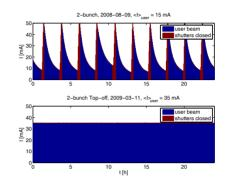
Figure 5: One day current history of two bunch operation in decaying beam mode and top-off. The average current is almost tripled (and shutters always stay open).
