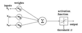
Figure 1: Schematic of an artificial neuron. The node receives inputs from other nodes which are multiplied by their respective weights and fed into the activation function.
