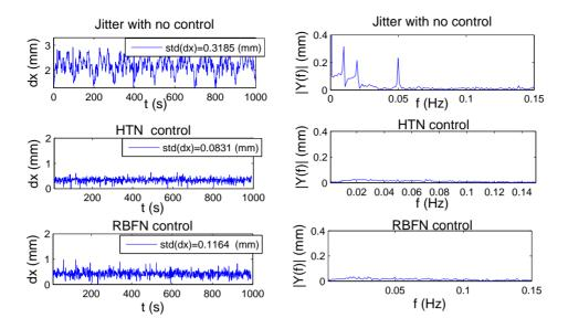
Figure 4: Example of real-time control over 1000 pulses, for voltage jitter of 0.06 kV amplitude and frequencies of 0.01 Hz, 0.05 Hz and 0.02 Hz. The upper plots give the recorded BPM readings (left) and the corresponding FFT (right) without control. The middle and lower plots give the BPM reading and the corresponding FFT when the control is operated with the HTN and RBF network, respectively.
