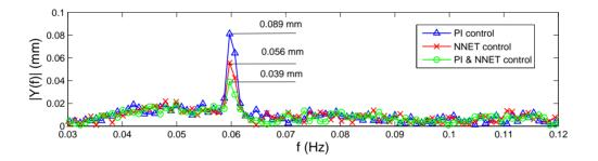
Figure 5: FFT for PI, NNET and combined controls, with jitter of 0.1 kV at 0.06 Hz.
