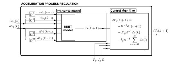
Figure 3: Control scheme consisting of a predictor (left block), connected in series to a control algorithm (right block). The predicted deviation dx(k + 1) is used by the control algorithm in the right block to compute forward (first term) and feedback (second and third terms) corrections, with user specified gains ( $P_g$  and  $I_g$ ) and sum range (R).
