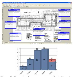
Figure 7: Examples for process support by information systems: Several reviewers provide mark-ups on a drawing in parallel (top), a report shows how many drawings have been received when and whether their processing is complete (bottom).
