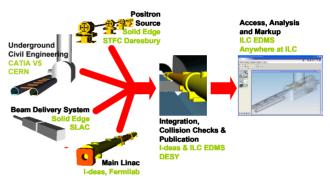
Figure 4: 3D CAD collaboration test scenario at ILC.
