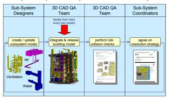
Figure 1: Process for 3D CAD collaboration (here: examples from XFEL).
