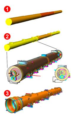
Figure 6: Lattice (1), accelerator made up of placeholders (2) and detailed component models (3). Placeholders link and decouple component design and facility planning.
