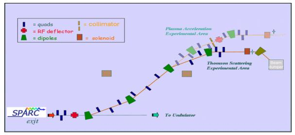
Figure 1: Lay-out of the dog-leg like electron beam line for the TS experimental area.
