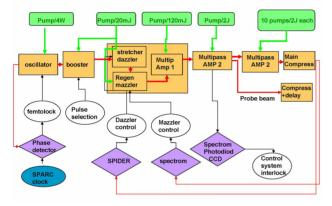
Figure 4: FLAME Laser layout.
