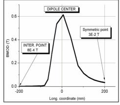
Figure 3:Last dipole field profile.
