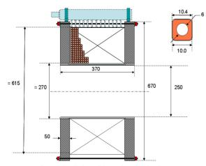
Figure 2: Solenoid engineered scheme.
