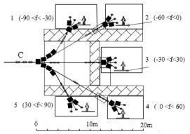
Figure 9: Scheme of New Planar System for ion beam with warm magnets with 5 treatment rooms in vertical plane and possible directions of irradiation for each room.
