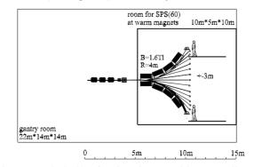
Figure 5: SPS(60) for ion beam with 7 small warm magnets.
