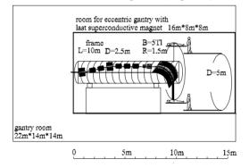
Figure 3: Eccentric gantry for ion beam with super conductive magnet (5Tl).
