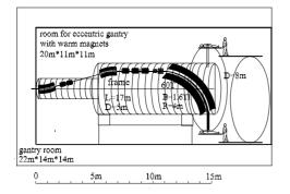
Figure 2: Eccentric gantry for ion beam with warm magnets.
