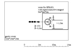
Figure 4: Simple Planar System SPS(60) for ion beam with superconducting magnet.
