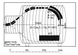
Figure 1: Gantry for ion beam with warm magnets.
