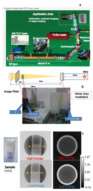
Figure 4: a) S-band Compton scattering source of NIAST, b) CT measurement set-up and c) CT reconstruction images of water-cell for the dual energies (30.8, 43.8 keV).
