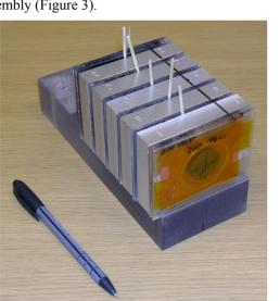
Figure 3: Shown above is the stack used for the sample irradiation. It consisted of 6 Tb foils, 5 Al degraders, and several Al beam monitors.
