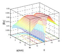
Figure 1: Magnetic field distribution of electron bunch varieties with frequency and observation angle  $\theta$  at  $0^{\circ}$  incidence angle.
