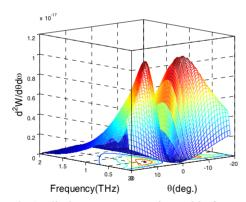
Figure 2: Radiation energy varying with frequency and observation angle  $\theta$ .
