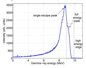
Figure 1: Measured energy spectrum of a gamma-ray beam produced by Compton scattering of a 466 MeV electron beam with a 789 nm Free-electron Laser beam at the High Intensity  $\gamma$ -ray Source (HI $\gamma$ S) facility. The gammaray beam is collimated by a lead aperture with a radius of 12.7 mm placed 60 m downstream from the collision point. After collimation, the gamma-ray beam is detected by a large volume 123% HPGe detector placed downstream 10 m from the collimator.
