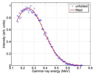
Figure 5: Illustration of the fitting on the high energy edge of the unfolded gamma beam spectrum. The non-linear least squares fitting method is applied to fit the model introduced in [2].
