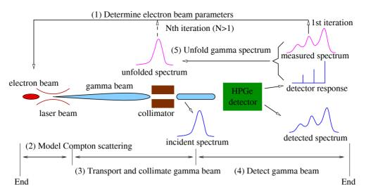
Figure 2: Illustration of the end-to-end spectrum reconstruction method to recover the energy distribution of a Compton gamma-ray beam. A few iterations are typically adequate to find a convergent energy distribution as well as the electron beam energy and energy spread.
