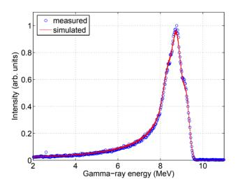
Figure 4: The simulated energy spectrum compared with the measured spectrum shown in Fig. 1.
