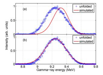
Figure 3: The unfolded energy spectrum compared with the simulated incident spectrum for a 9 MeV HI $\gamma$ S beam. Two iteration is needed in order to find a convergence between the unfolded spectrum and simulated spectrum. (a) First iteration; (b) second iteration.
