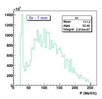
Figure 4: Momentum distribution for muons produced by a 7 mm graphite target.
