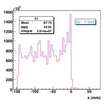
Figure 7: Histogram of the x-coordinate of the pion decay for muons extracted from the graphite target. The muon beamline window is at x=-150 mm. The peak around x=0 corresponds to pions decaying at rest in the target.
