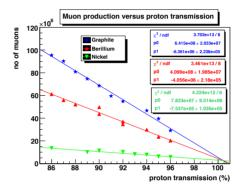
Figure 3: Muon production as a function of proton transmission for graphite, beryllium and nickel targets (momentum is in the range 25-250 MeV/c).
