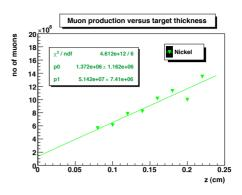
Figure 2: Muon flux dependence on target thickness for nickel (momentum is in the range 25-250 MeV/c).
