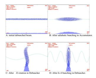
Figure 2: Bunched beam preparation for the Mu2e experiment. The dots are particle distributions in phase (horizontal,  $\pm 180^{\circ}$  or  $\sim \pm 0.85 \ \mu sec$ ) and energy (vertical,  $\pm 200 \text{ MeV}$ ) phase space, with histograms shown along the bottom edge. See [4] for details.
