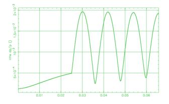
Figure 3: Resulting rms  $\Delta p/p vs.$  time in seconds following Recycler injection. Beam is rotated and captured into four buckets. The half-rotation time is 12 msec allowing extraction one-by-one as the momentum spread reaches its peak (pulse length is at its shortest).
