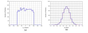
Figure 8: Uniform and Gaussian distribution with  $\sigma_E$ = 200 keV in (a)  $\Delta \phi$  and (b)  $\Delta E$  spaces.
