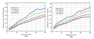
Figure 5: Emittances as a function of injection turns in (a) horizontal and (b) vertical directions.
