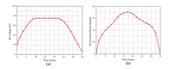
Figure 6: Ramping of (a) RF voltage and (b) the synchronous phase.
