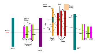
Figure 2: Layout of the injection system for PEFP RCS.
