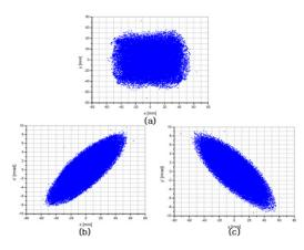
Figure 3: Particle distribution after injection in (a)x-y space, (b) x-x' space, and (c) y-y' space.
