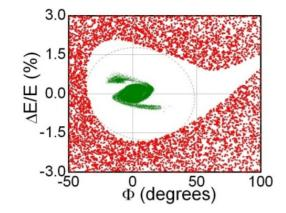
Figure 7: Longitudinal acceptance of the 1.3 GHz elliptical accelerating structure at  $\sim$  156 MeV (white) together with the matched input beam phase space (green).
