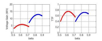
Figure 6: Voltage gain (left) and transit time factor (right) for the alternative accelerating lattice.
