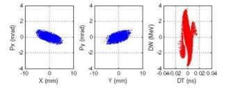
Figure 9: Horizontal (left), vertical (middle) and longitudinal (right) phase spaces at the exit of the alternative lattice, at a beam energy of ~1.2 GeV.
