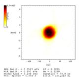
Fig. 3: Tomographic image of the LHC Probe beam in the PSB; intensity 5.2×10<sup>9</sup> protons, momentum spread ~10<sup>-3</sup>, bunch length ~70 ns and longitudinal emittance ~0.2 eVs.
