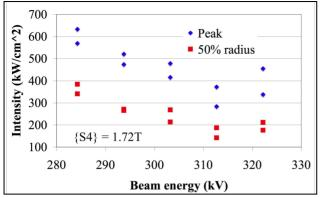
Figure 6. Parametric scan of beam intensity with beam energy.
