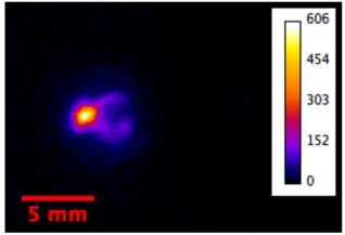
Figure 7. Intensity map of the beam distribution at the target plane. Units are  $kW/cm^2$ .
