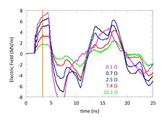
Figure 3: The FAST's on-axis accelerating field waveform with various SiC on-resistance.
