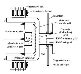
Figure 5: Layout of proton injector and FAST.
