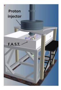
Figure 4: Proton injector and FAST test stand.
