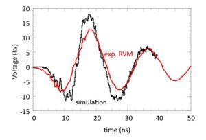
Figure 2: The FAST's accelerating voltage pulse.
