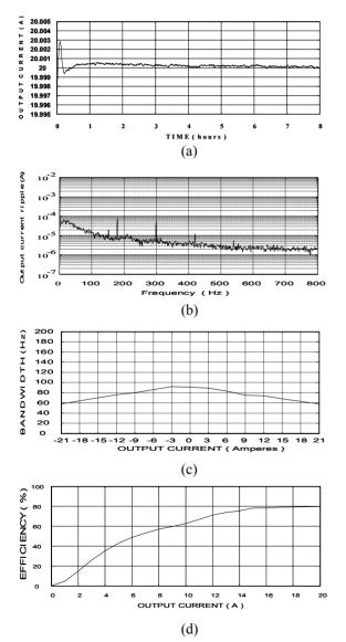
Figure 3: The performance of MCOR30 power module (a) Output current stability, (b) Spectrum of output current ripple, (c) Frequency response bandwidth (d) Efficiency.
