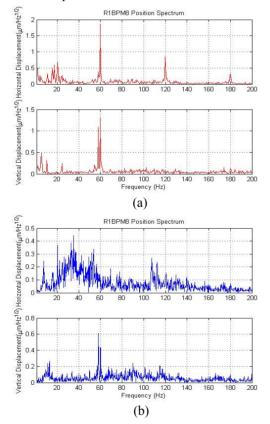
Figure 4: Spectrum of vertical and horizontal beam position displacement variation (a) After 1st phase installation of MCOR30s (b) After 2nd phase installation of MCOR30s.
