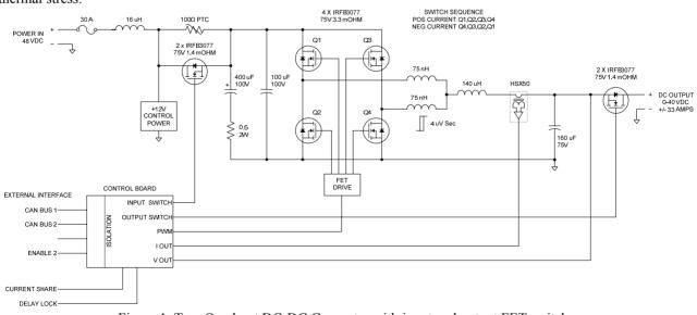
Figure 1. Two Quadrant DC-DC Converter with input and output FET switches
