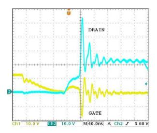
Figure 2: FET Diode Turn off 30 amps
