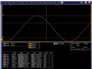
Figure 2: Actual output current waveforms of dipole power converter (two traces are overlapped) at maximum extraction energy (2.5 GeV).
