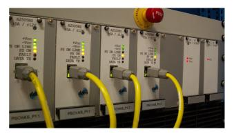
Figure 5: Crate containing 4 A2505 units with auxiliary "bulk" power supplies.
