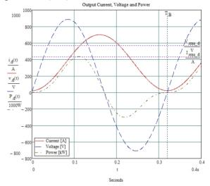
Figure 1: Ideal output waveforms for each dipole power converter at maximum extraction energy (2.5 GeV).
