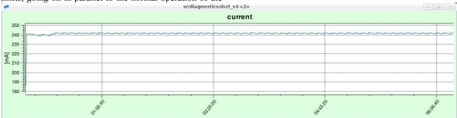
Figure 3: "Frequent Injection" tests at Elettra – for more than 5 hours the Storage Ring current is kept at 242 mA.
