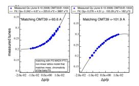
Figure 1: Example of non-linear chromaticy measurement for one of the MTE octupoles.
