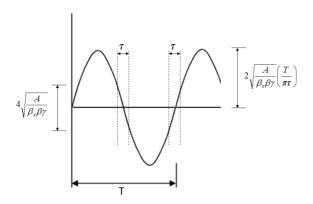
Figure 3: Concept for the AC dipole system. Because beam is transmitted at the node, the system only needs to run at half the bunch frequency. However, producing a short transmission window requires the system to run at a higher amplitude than would otherwise be needed.
