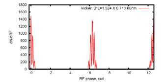
Figure 8: Time distribution of surviving beam, plotted as a function of the phase corresponding to the bunch frequency (twice the AC dipole phase). Pseudo-bunch separation is approximately 50 ns.
