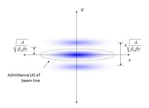
Figure 4: Effect of the AC dipole field in phase space. Beam line admittance A is indicated by the ellipse.
