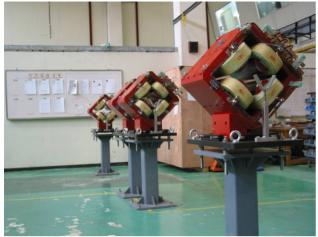
Figure 5: quadrupole magnets.
