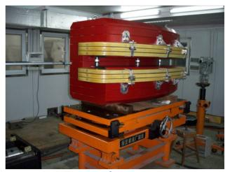
Figure 4: 45° dipole magnet.
