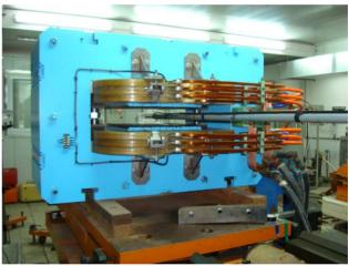
Figure 3: AC magnet for beam distribution.
