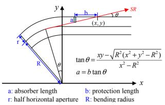
Figure 6: Sketch drawing of the synchrotron radiation emitted from the dipole magnet and blocked by the photon absorber.
