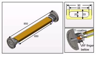
Figure 4: Configuration of TPS ceramic chamber.
