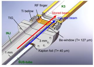
Figure 2: Cutaway view of the assembly of K3, INJ and the SUS-tube.
