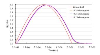
Figure 5: Attenuated fields inside the ceramic chamber relative to the external half-sine  $(5.18 \,\mu s)$  kicker field.
