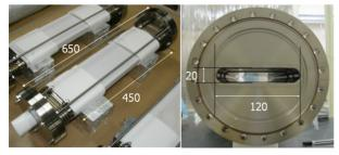
Figure 3: TLS ceramic chamber.
