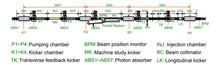
Figure 1: Layout of the TPS injection section with diagnostic components and pulsed magnets.
