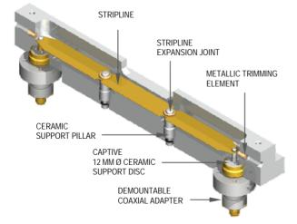
Figure 9: Planar test assembly / Cut-away view.
