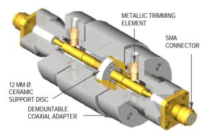
Figure 3: Coaxial Test Assembly / Cut-away view. Accelerator Technology - Subsystems
