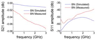
Figure 4: Coaxial Test Assembly / S parameters.
