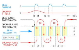
Figure 1: Slow-wave structure design.
