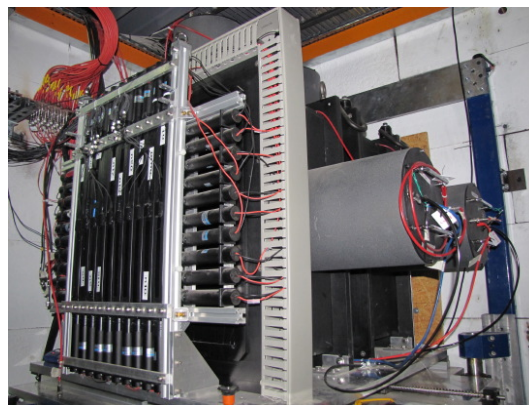
Figure 2: X/Y planes for TOF0 station. Each bar assembly is 4 cm wide. (The CKOV detectors are behind the TOF0)
