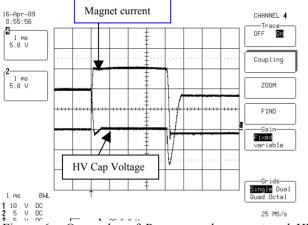
Figure 6: One pulse of Power supply current and HV Capacitor voltage
