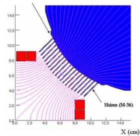
Figure 3: Modeled field with shims added.
