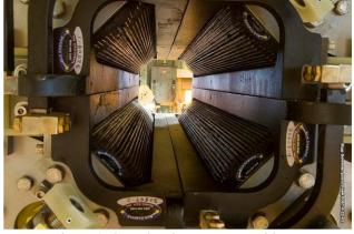
Figure 4 Completed Magnet assembly
