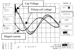
Figure 2: Ring Test showing response to impulse voltage. #1- Cap Voltage/200;
