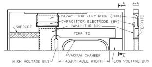
Figure 1: Cross-section of the kicker magnet; one quarter of one cell is shown.
