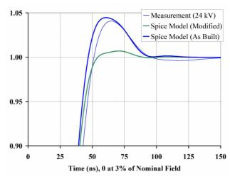
Figure 3: Calculated and measured integrated magnetic field; model with reduced capacitance.
