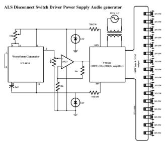
Figure 2: High voltage insulated driver AC power system.
