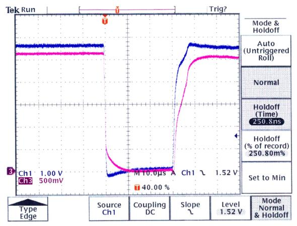
Figure 4: Oscilloscope output of the voltage on the first and second switch module during turn-on/turn-off cycle (V=7kV; I=35A).
