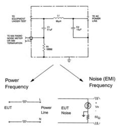
Figure 2: Shows the LISN internal structure and Vn, it obtains conducted voltage noise generated by LISN.
