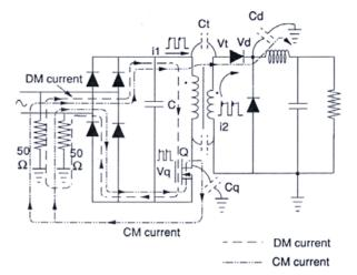
Figure 6: The noise source and coupling Path.
