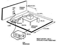
Figure 1: Indicates the lab Equipment under test the connection of LISN diagram.
