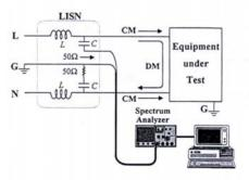
Figure 3: It shows the detail of LISN internal structure and with EUT connecting diagram and notice path loop.
