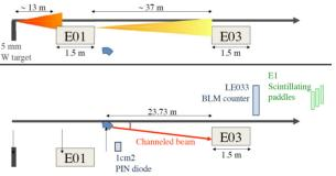
Figure 1: Layout of the Tevatron E0 region with tungsten target (top) and crystal (bottom).
