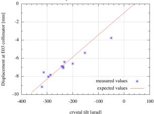
Figure 4: Displacement of channeled beam from beam core at E03 vs. crystal angle.
