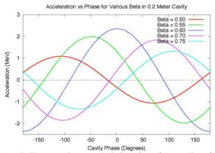
Figure 3. Energy gain versus relative phase for a cavity of length 0.2 m.
