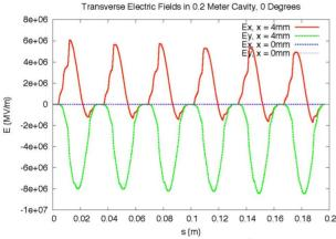
Figure 6. Vertical and horizontal electric fields seen by particle at  $\beta = 0.6$  and 0° phase for x = 0 mm and for x = 4 mm.
