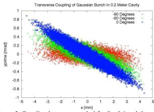
Figure 5. Coupling between x and y' for  $\beta = 0.6$  and three different phases.
