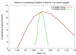
Figure 2. Maximum accelerating gradient versus  $\beta$  for cavities of length 0.2 m and 1.0 m.
