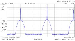
Figure 1: Schottky spectrum with coherent lines.
