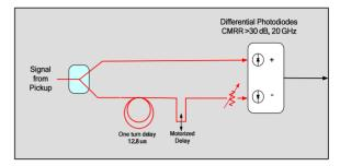
Figure 6: Notch filter for longitudinal cooling
