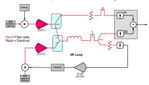
Figure 8: Filter with IIR loop for transverse cooling to remove common mode signal
