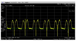
Figure 7: Longitudinal Schottky spectrum filtered by cooling filter with notches
