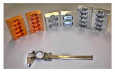
Figure 11: Three kicker cavities. Left is copper plated aluminum.
