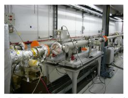
Figure 4: The two long-range beam-beam wires in the RHIC tunnel during installation.
