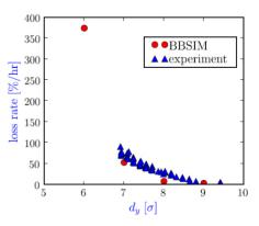
Figure 7: Comparison of measured and simulated beam loss rate as a function of distance between wire and and beam. Experiment with gold beam at store, wire strength of 125 A m [24].
