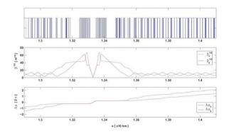
Figure 2: LHC IR lattice functions. At s = 13.433 km, with approximately equal transverse  $\beta$ -functions, a long-range wire compensator or electron lens could be placed.
