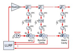
Figure 1: RF control block diagram for HINS.
