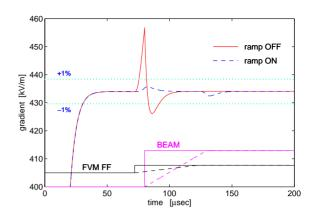
Figure 4: Beam compensation with FVM transient response for HINS cavity no. 6.
