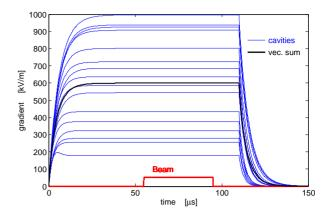
Figure 5: Beam compensation with klystron FF and FVM.
