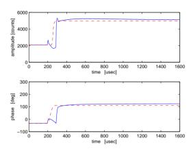
Figure 3: Amplitude and phase response of the FVM to a 3dB attenuation request.
