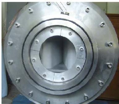
Figure 7: The new dumper with two slope plates.
