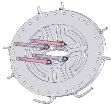
Figure 5: The mechanical drawing of the coupling plate, on which the rods are installed and embedded with water-cooling channels.
