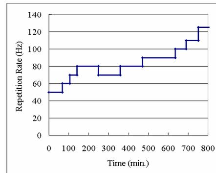
Figure 8: Time diagram of the RF conditioning.
