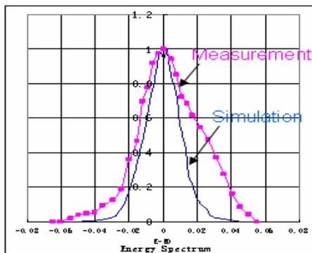
Figure 3: The measured energy spectrum is similar to the simulation result from PARMTEQM
