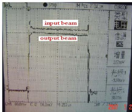
Figure 4: The output pulsed beam current is about 44.5mA with a beam transmission about 93% and beam duty factor of 7.15%.
