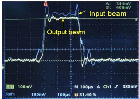
Figure 2: A beam transmission about 92% with an input beam current of 44mA and a beam duty factor of 0.5% is got in the initial beam commissioning.
