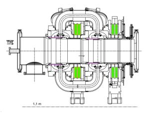
Figure 1: Side-view of planned ferrite loaded rf cavity for PAMELA.
