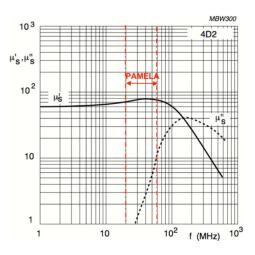
Figure 2: Frequency dependence of permeability of Ferroxcube 4d2[10].  $\mu'_s \mu''_s$  mean real part and imaginary part of complex permeability, respectively.
