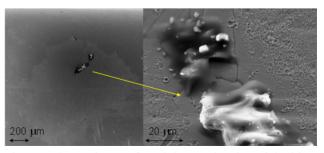
Figure 5: SEM photos of a calcium and carbon rich object on iris 12 of the CERN T18 structure.
