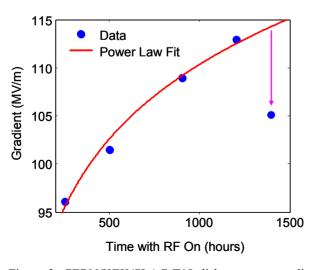
Figure 3: CERN/KEK/SLAC T18 disk structure gradient over time with 230 ns pulses and a breakdown rate of 2e-6 pulse per meter.
