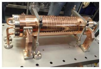
Figure 4: Photo of the T18 CERN structure mounted on the top plate of a vacuum can.
