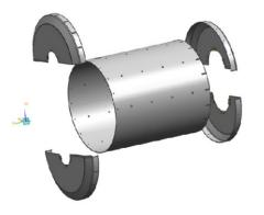
Figure 3: The parts of the cavity magnetic shield.
