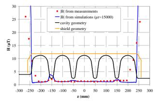
Figure 5: Magnetic field on the cavity surface from simulations and field map measurements. The black solid line indicates the cavity geometry and the orange line shows the magnetic shield geometry.
