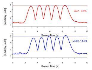
Figure 7: Field flatness after final integration of the two cavities, Z501 and Z502.
