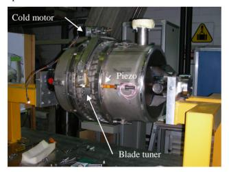
Figure 1: The TRASCO cavity equipped with Helium tank and blade tuner in the warm test stand.
