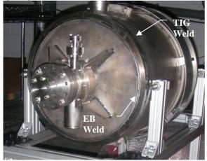
Figure 6: Cavity-Tank welded connection.
