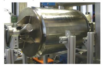
Figure 4: The shield around the cavity.
