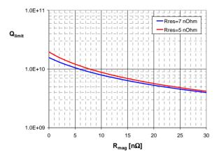
Figure 2: Cavity Q as a function of the contribution to surface resistance by trapped magnetic flux ( $R_{mag}$ ).
